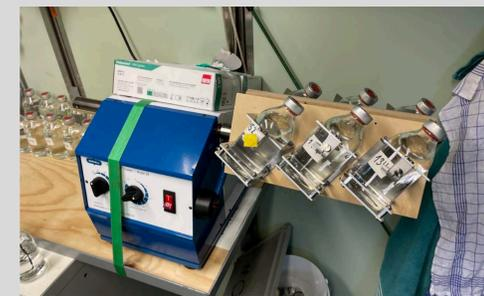
To ensure a consistent mixing procedure, a shaker is used to shake the sampling bottles right before they are measured with the OPS.
