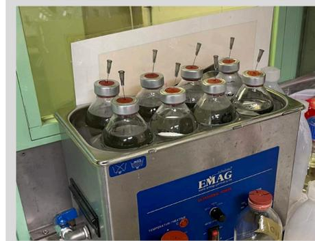
Bottles in temperature bath with injection needles stabbed through the lid for degassing. Needles should be applied only for a few seconds, to minimize evaporation.
