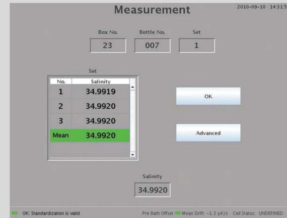
Left picture: Display of a typical result shown on the touch-screen display after finishing the measurement of a water sample bottle. The top row gives the sample number as given by the operator at the beginning of the measurement cycle. Below the three measured salinity values as well as the mean are listed. Those results are automatically logged in a text file. The advanced mode can be used by the operator to get more information on the status of the conductivity cell.
