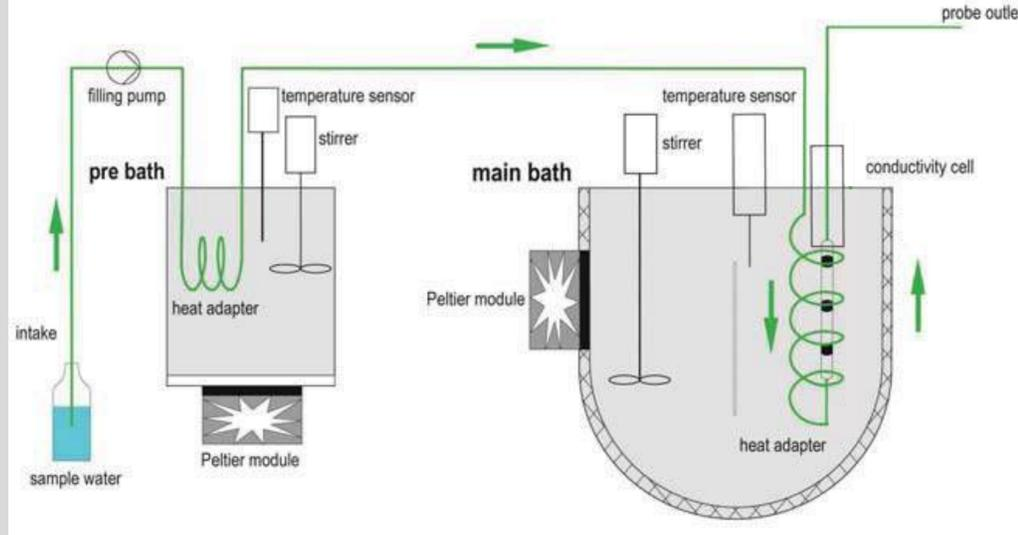
Schematic showing the main elements of the Optimare Precision Salinometer
