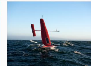
Figure 2. Saildrones – autonomous sailing drones – are used as a tool to provide high quality oceanic and atmospheric observations.
