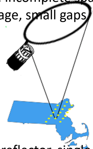
Large reflector, single feed: incomplete spatial coverage, large gaps.
