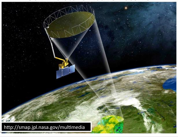
Orbit Altitude: 685 km. Inclination: 98 deg. Local ascending/descending time: 6 PM/AM. 8-day repeat orbit.
