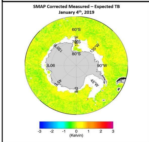
**ABOVE:** Figures depicting the 8-day averaged measured minus expected (i.e., calculated from a radiative transfer model) brightness temperatures from SMAP (left) and AMSR-2 (right) centered on January 4<sup>th</sup>, 2019 around Antarctica.
