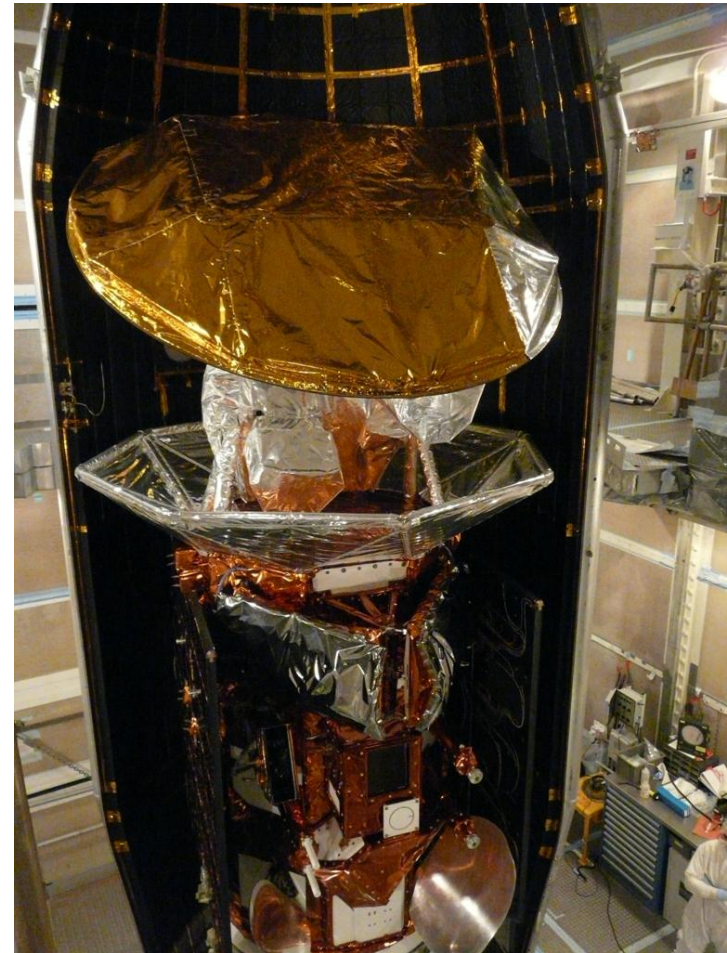
Aquarius/SAC-D observatory ready for closure of the fairing
